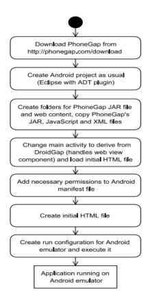
Figure 4: Procedure of Installation and First Application Run Using Phone Gap [11]
